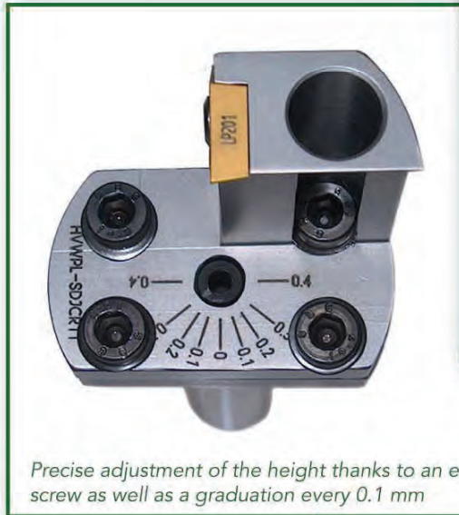
Fitting with Bimu 040 / 400 inserts
