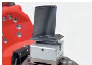
SX-Rotary A/B axis • High precision A/B axis – A rotary axis \pm 115^\circ – B rotation axis 360^\circ – Direct axis measurement – Designed for 3R or EROWA chuck – Resolution 0.0001 degrees – Workpiece holder internal flushing
