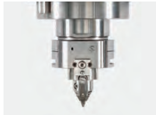
SP06 • High precision automatic electrode feeding collet – Runout adjustment – Internal high pressure flushing – Diameter range \varnothing 0.05 to \varnothing 1.5 mm – Up to \varnothing 0.99 it fits to clamping range of 0.04 mm
