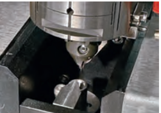
SX-Laser measuring • Laser for electrode diameter/profile measuring for SX-Ariane – Resolution of 0.10 \mu\text{m} – Minimum measurement of 0.005 mm
