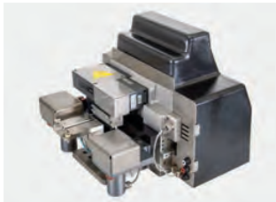
SX-Ariane • Wire Dress unit – Designed to produce micro-electrodes for micro-holes and micro-forms down to \varnothing 10 \mu\text{m} – Wire \varnothing 0.10 and 0.20 mm
