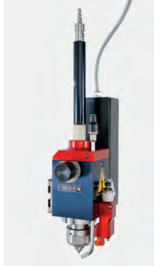
SX-A344L • Automatic electrode feeding and wear compensation spindle – Internal high pressure flushing – 3R chuck – Roundness \pm 1 \mu\text{m} – Speed max 850 rpm – For collets SP06, SP12 and SP-MDC
