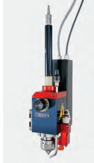
SX-C-A344L • Indexable automatic electrode feeding and wear compensation spindle – Internal high pressure flushing – 3R chuck – Speed max 600 rpm – For collets SP06, SP12 and SP-MDC
