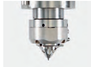
SP12 • High precision quick change automatic feeding collet – Runout/tilt adjustment – Internal high pressure flushing – Diameter range \varnothing 0.05 to \varnothing 1.5 mm – Up to \varnothing 0.99 it fits to clamping range of 0.04 mm
