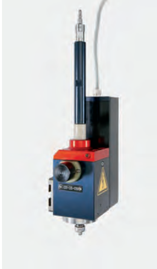
SX-ROT • Manual electrode feeding spindle – Internal high pressure flushing – 3R chuck – Roundness \pm 1 \mu\text{m} – Speed max 850 rpm – For collets SP02, SP03 and SP04
