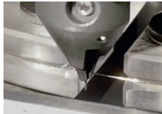
SX-Ariane • Wire Dress unit – Designed to produce micro-electrodes for micro-holes and micro-forms down to \varnothing 10 \mu\text{m} – Wire \varnothing 0.10 and 0.20 mm
