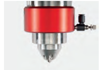
SP-MDC • Automatic multi diameter collet – Internal high pressure flushing – Diameter ranges \varnothing 0.2 to 1.0 mm, \varnothing 0.5 to 1.5 mm and \varnothing 1.0 to 4.0 mm
